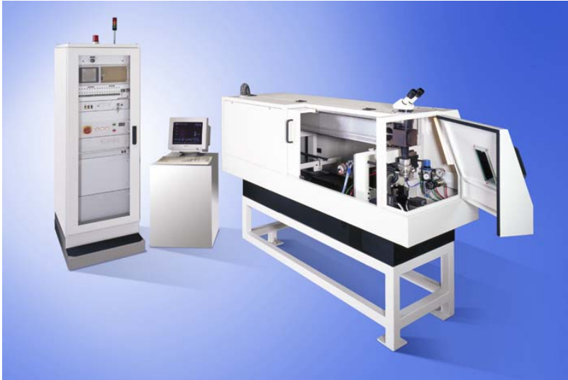
Fig. 1 The StarTube is a fully automatic laser cutting system
