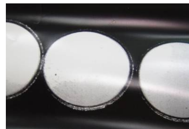
Picture 1: Ablation with a round 600 µm fiber = 0,283 mm 2
